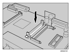
Insert the DIMM into the slot, and push it down until it clicks. If the DIMM is not set in the correct way, it does not click.
