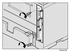
While aligning the power cord to the left side groove of the Duplex Unit, slide the Duplex Unit in until it is connected to the printer.
