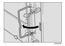
Pull the handle and slide the controller board out slowly.
